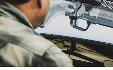
discharge had previously been the job of the safety mechanism. The quandary was a light trigger pull improved accuracy but made it easier for jarring to release the sear causing accidental discharge but heavier trigger pull affected accuracy. and still doesn't guarantee accidental discharge prevention.
