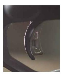
Enter AccuRelease, a unique safety mechanism that sets AccuTrigger apart. AccuRelease, in simple terms, is a physical block in the path of the sear; think of it as a seesaw mechanism. A blade through the trigger shoe acts much like a two-stage trigger; it must first be depressed which lowers the seesaw block out of the way of the sear before the trigger is pulled. Even if the trigger is hit from the side, for instance when you
